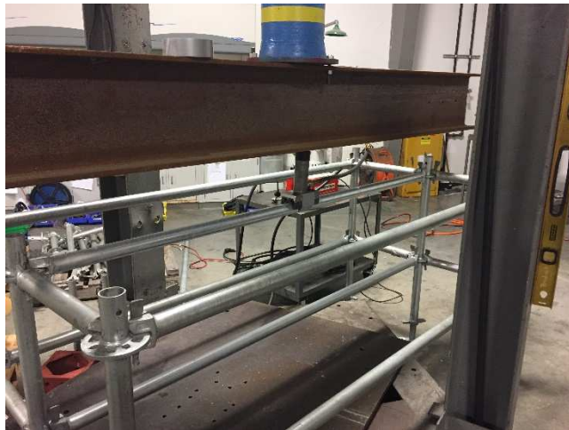
Point Load Test
