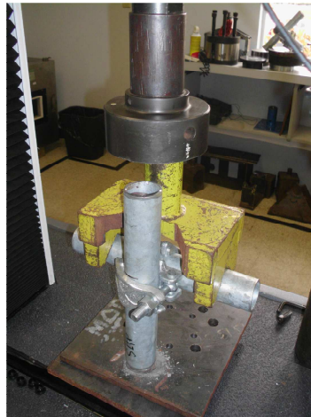
Load method for right angle and swivel couplers
