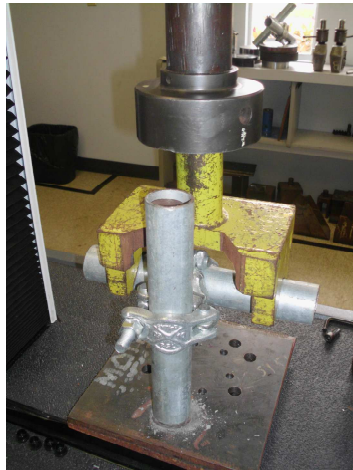
Load method for right angle and swivel couplers
